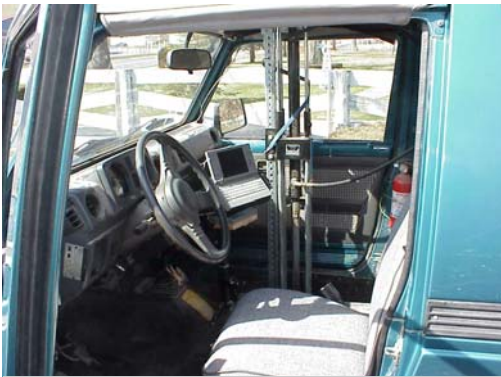
The high tech soil probe and its GPS system with computer monitor are mounted on the passenger side of this specially modified vehicle.
